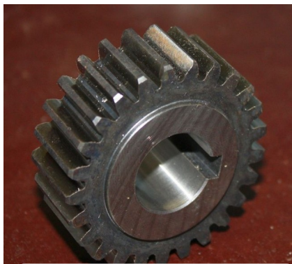
View of the prepared gear flank (brown "12 o'clock")
